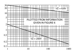
Fig. 6-PEAK SURGE CURRENT VERSUS PULSE WIDTH(SEE NOTE 3)
